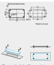
The mounting hole of the mounting cabinet can be temporarily sealed. Applicable to the installation hole which has been opened, The case where the connector is not installed
